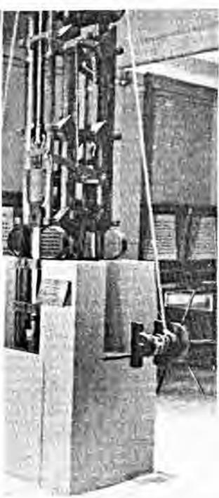
*Fig. 15.—Reconstruction of a coin-stamper designed by Leonardo da Vinci. It emphasizes the introduction of mechanization in coining techniques. The machine was built for the Smithsonian Institution in the laboratories of the International Business Machines Corporation by Dr. Roberto Guatelli*
